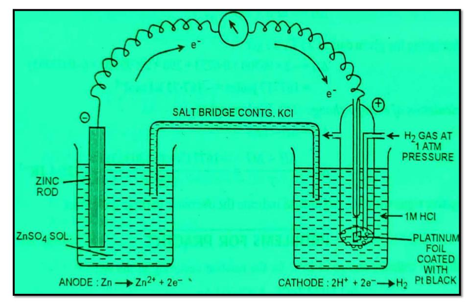
Measurement of E<sup>o</sup> using S.H.E.
