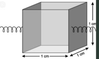
Hence Specific conductivity is defined as conductance of the solution of 1 cm length and having 1 sq.cm as the area of cross section or it is the conductance of 1cm cube of the solution of the electrolyte.
