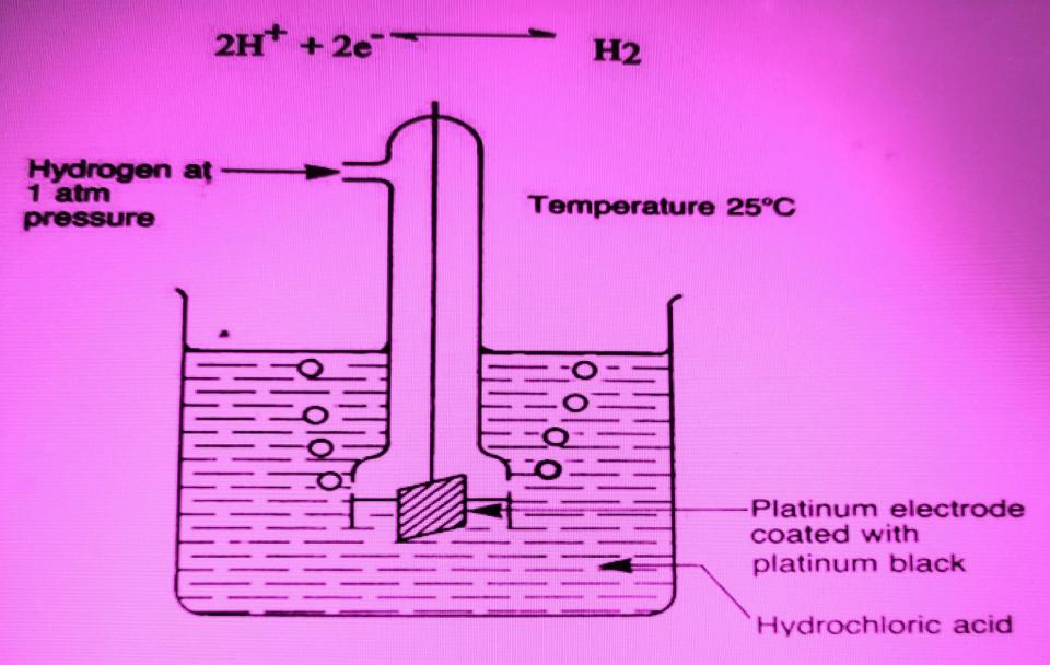
A standard hydrogen electrode (S.H.E.)
