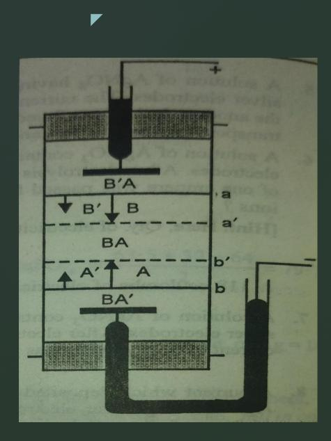
Moving Boundary method for determination of Transport Number.
