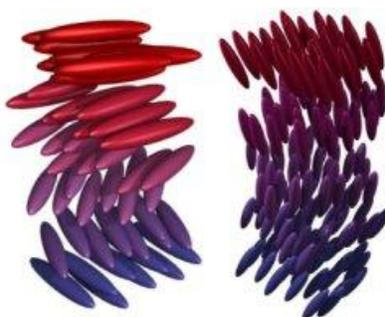
**Fig. (c)** Schematic of ordering in chiral liquid crystal phases. The chiral nematic phase (left), also called the cholesteric phase, and the smectic C\* phase (right).
